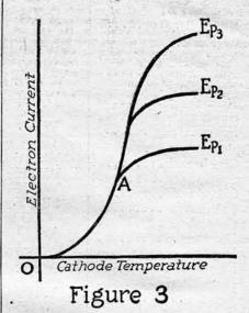
etc., may be taken to represent the rate of vaporization of electrons with varying temperature.
