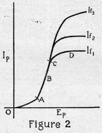
2 the ratio  $E_p\colon I_p$ , where  $E_p$  represents the voltage across battery (B) and  $I_p$  the current flowing through the external circuit (Figure 1) from the anode (P) to the cathode (F).
