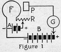
In order to determine definitely just what does occur under given conditions, we will connect a two-electrode tube as shown in Figure 1. Here the cathode (F) is heated by current supplied by battery (A), and (P) is the anede. The anode (P) and the cathode (F) are connected together through a galvanometer (G) and an anode battery (B). The temperature of the filament may be regulated by varying the heating current by means of the resistance (R).
